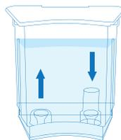
Water is pumped into the filters through the inlet on the right. Water is recirculated back into the tap tank from the inlet on the left.
