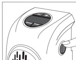
2. Press “On/Off Switch” on side of the unit to “On” position to turn on the heater.
